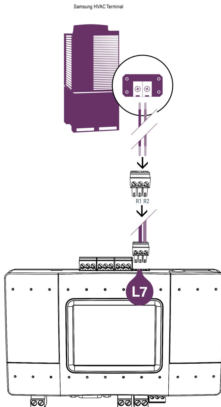
The above connection would allow you to control up to 64 indoor units from a single connection to the outdoor unit. Refer to the manual of the HVAC unit for recommendations on cable used for this connection. For example a Samsung VRF unit recommends a cable gauge of 0.75mm to 1.5mm.
