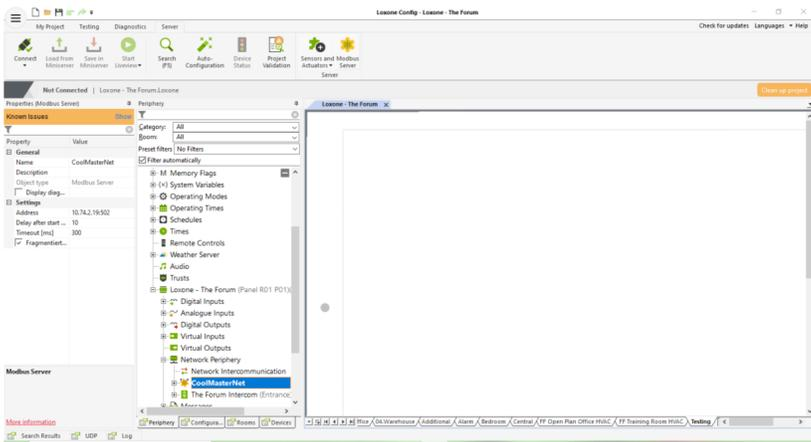
Select 'Network Periphery' in Config, then at the top ribbon click 'Modbus Server'. This will add the Modbus server to the periphery list. Then fill out the parameters for the IP address of the CoolMasterNET and the port (default port is 502)
