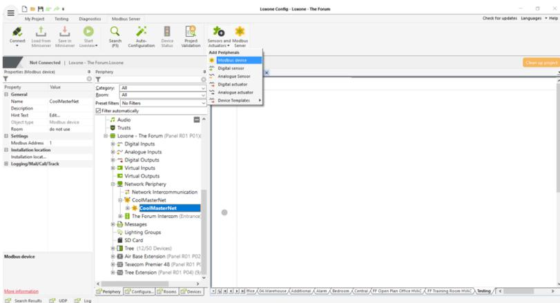
Select the Modbus Server in the periphery list and then select 'Sensors and Actuators' from the ribbon. Click 'Modbus device' this will create an address beneath the server. The default address will be 1.
