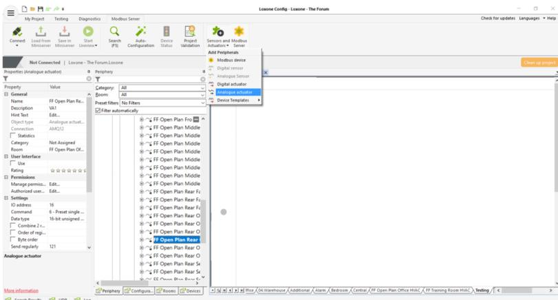
Select the Modbus device then select 'Sensors and Actuators' from the ribbon. Create inputs and outputs as required. We recommend all sensors and actuators be 'Analogue' to be able to correctly set the command type.
